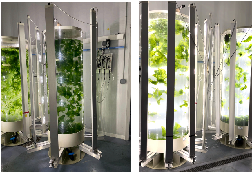
Figure 3 - 500L PBRs (left) and 1000L PBRs (right)
