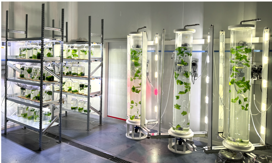
Figure 2 - 4L PBRs on culture shelves (left) and 100L PBRs (right)
