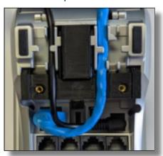
3. When the cables are properly seated in their ports, gently pull on the cables to remove any excess cable that is higher than the plane of the T bracket.
