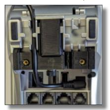
2. Insert the Ethernet cable in the terminal's cable guide on the right and connect it to the **LAN** port.
