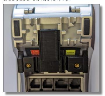
2. Slide the T bracket up by pushing it from the bottom towards the top of the terminal.
