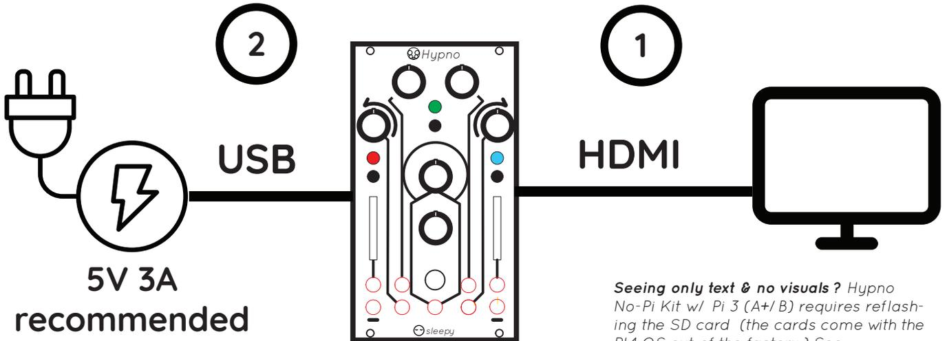
*Seeing only text & no visuals? Hypno No-Pi Kit w/ Pi 3 (A+/ B) requires reflashing the SD card (the cards come with the Pi4 OS out of the factory.) See docs.sleepycircuits.com for instructions.*
