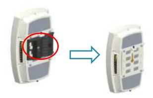
2. Fit the CPE on the wall, and mark the drilling locations.
