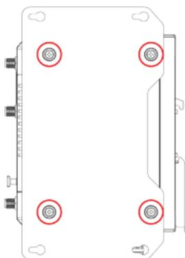
**STEP 2:** Use the CCG-1500 Series device with the wall mount plates attached as a guide to mark the correct location of the four screws. The heads of the screws should be less than 6.0 mm in diameter, the shafts should be less than 3.5 mm in diameter, and the length should be at least 10 mm in diameter.
