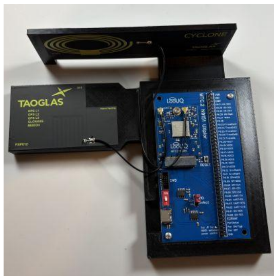
The UXplor QuickStart (MTC2-N9151) kit: MTC2-N9151 mounted on the UXplor carrier board, wired to the Taoglas GNSS antenna (left) and Cyclone NTN antenna (top).
