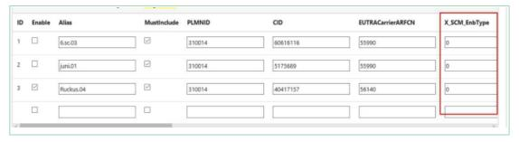
The PCI range of different type eNB will need to be configured if using ANR to add neighbor cell. Visit "FAPControl" page under "FAPService" group to configure X\_000E8F\_CSGSmallCellPCIStart and X\_000E8F\_CSGSmallCellPCIRange. In the following figure, PCI range of Home eNB is from 485 to 503 (both 485 and 503 are included).
