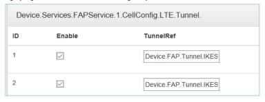
TunnelRef: set 1st one to Device.FAP.Tunnel.IKESA.1 and set 2nd one to Device.FAP.Tunnel.IKESA.2.
