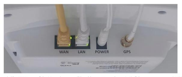
Step 2. The WAN port of the Moso Canopy will be able to get one dynamic IP if the router supports DHCP server. Or refer to "Configure Device's Network" section to setup the WAN port of the Moso Canopy.
