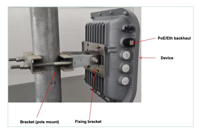
Step 4: Install the RJ45 Cable, PoE++ in (45W / 1 Gbps)
