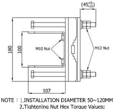
NOTE : 1.INSTALLATION DIAMETER 50~120M 2.Tightening Nut Hex Torque Values: M10 :32~40 N.m M12 :57~75 N.m
