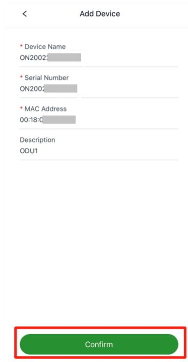
Step 3: After scanning the code successfully, configure the name, serial number, and description information of the device.
