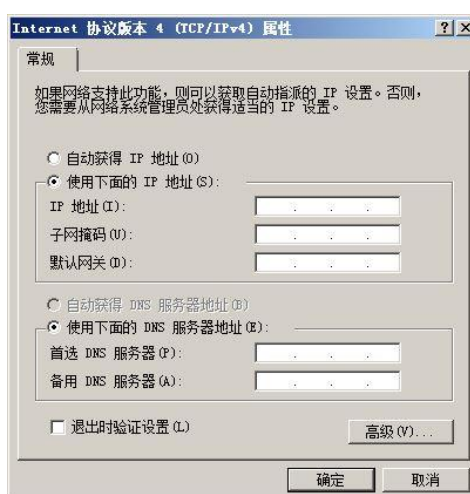
Figure 3-2 setting the client IP address
